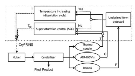
Figure 2: Schematic of the Active Polymorphic Feedback Control (APFC) approach. Raman spectroscopy is used to detect the presence of the undesired form (P) using a calibration-free approach; ATR-UV/Vis is used to measure the solute concentration (C) and perform SSC using a calibration-based approach to determine the setpoint for the temperature controller,  $(T_{sp})$  (17).
