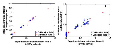
Figure 1: PLSR and PCR calibration and validation concentrations of form II with data obtained from the DoE.
