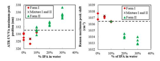
Figure 6: (a) UV/Vis and (b) Raman OABA peak positions in undersaturated conditions and corresponding polymorphic outcomes for cooling crystallization experiments. Two different cooling rates (-1 and -0.5 °C/min), two level of saturation temperature (30 and 40 °C) and several different solvent compositions (from 0 to 25% IPA in water) were used.
