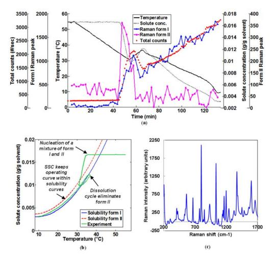
Figure 3: Results of the APFC approach applied to an unseeded experiment: (a) time evolution of temperature, concentration, Raman signals for form I and II and total counts/s from FBRM; (b) operating curve in the phase diagram; and (c) Raman spectrum for the final dried solid material confirming pure form I.
