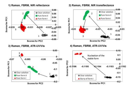
Figure 4: Plots of PC1 vs PC2 for clear solution, pure form I and pure form II in several experiments conducted using different collections of PAT tools. The graphs show the ease of detecting crystallization phenomena such as nucleation and polymorphic transformations.
