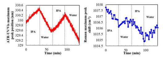
Figure 5: UV/Vis (a) and Raman (b) peak shifts during continuous alternate addition of water and IPA to an unsaturated solution of OABA in water (0.011 g OABA/g water). The flowrate was of 2 mL/min and water and IPA were pumped alternatively for about 30 min, twice.
