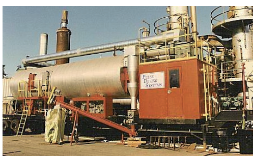
Figure B2 Mobile pulse combustion dryer with evaporation capacity of 2000 kg water/hr (courtesy of Pulse Drying Systems, Inc., Portland, OR, USA)
